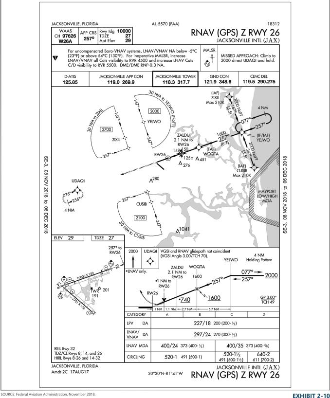
**INSTRUMENT APPROACH PLATE** RUNWAY 26 AREA NAVIGATION GLOBAL POSITIONING SYSTEM
