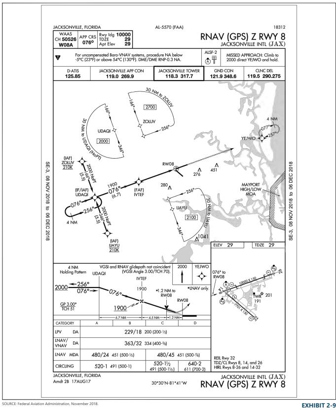
INSTRUMENT APPROACH PLATE RUNWAY 8 AREA NAVIGATION GLOBAL POSITIONING SYSTEM
